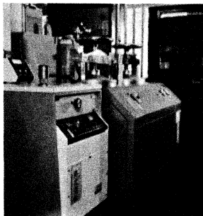
Fig. 4 Helium leakage tester
